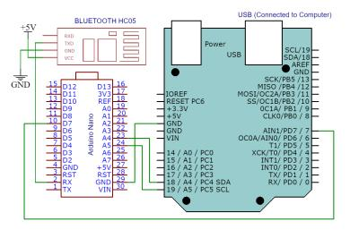
Figure 5. Circuit diagram of the receiver unit.
