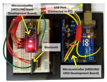
Figure 6. Prototype of the receiver unit.
