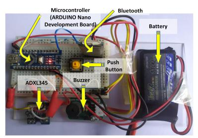
Figure 4. Prototype of data acquisition and transmitter unit.
