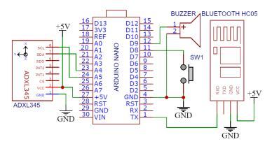
Figure 3. Circuit diagram of data acquisition and transmitter unit.
