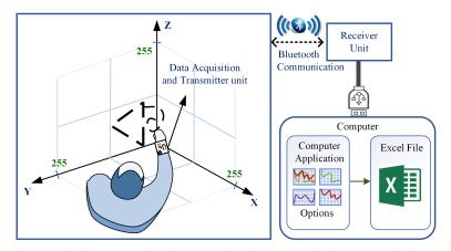
Figure 2. Block diagram of data acquisition system.
